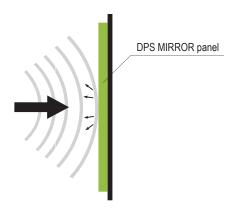
reduction of sound wave reflection when using DPS MIRROR Acoustic panels
